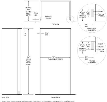
NOTE:  $3^{1}/2^{\circ}$  (89) finished returns and shaded areas will be visible and should be finished to match cabinetry. Shaded line represents profile of unit with  $3^{1}4^{\circ}$  (19) panel.
